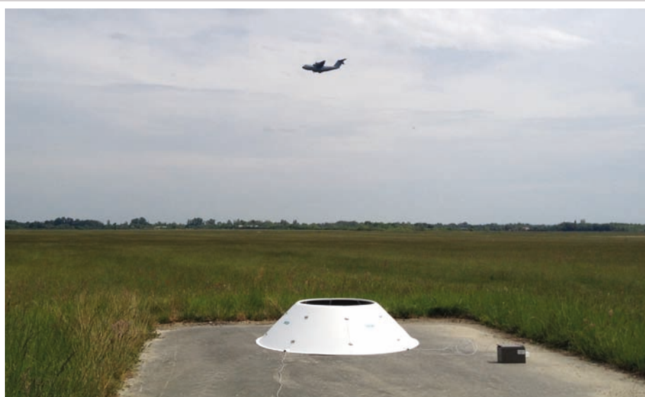
PA0 Sodar with its standard extra acoustic enclosure made of 8 easily assembled sections
